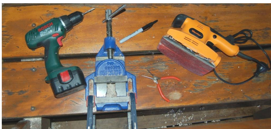
Figure 5. Equipment needed to make drilled wood blocks for resin bee nests. Cordless drill to drill smaller holes, vice, marking pen, needle nose pliers and sander.
