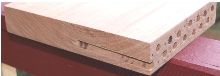
Figure 3. Burrows drilled across the wood grain.
