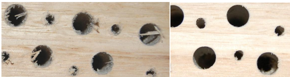
Figure 9. Drilled burrows with burrs at entrances (left) and holes with burrs removed and sanded smooth (right).
