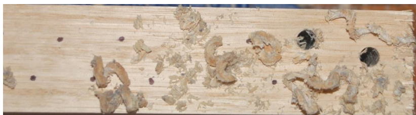
Figure 7. Holes cleared of wood chips.
