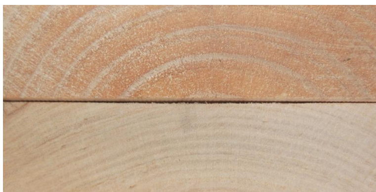
Figure 2. Soft wood (top) compared to hardwood (bottom).
