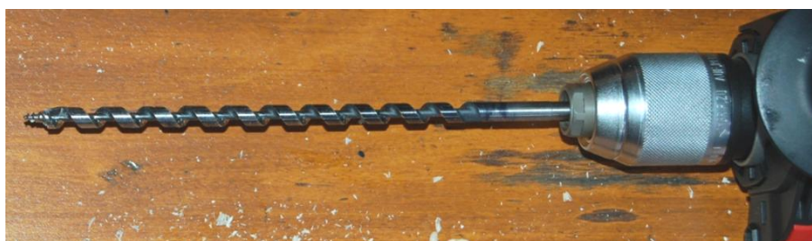
Figure 4. Long auger bit is best for drilling hardwood.
