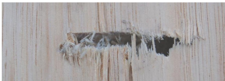
Figure 8. Side of block ripped open by crooked drill bit.
